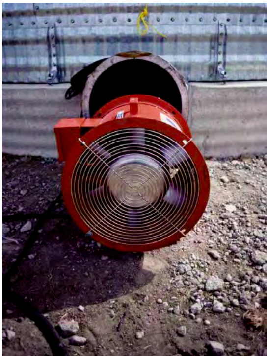
Photo 12: Aeration fan ready to be mounted
