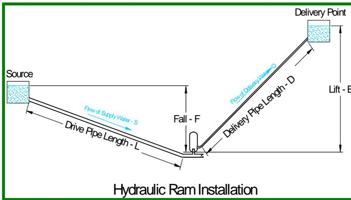
The discharge that can be delivered to the delivery point can be approximated from the following equation:
