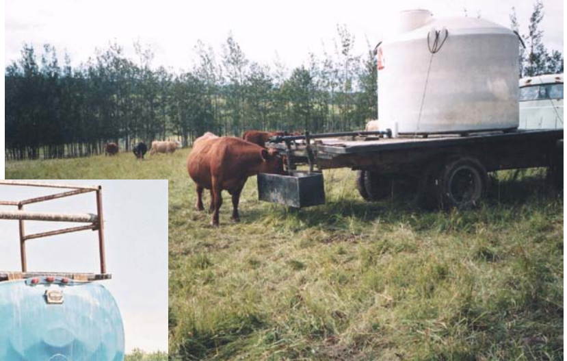
Truck-Mounted Water Tank With Integrated Trough
