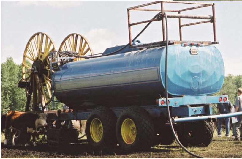
Trailer-Mounted Water Tank With Distribution Hose
