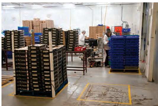
Visual management - floor outlines and hanging signs.
