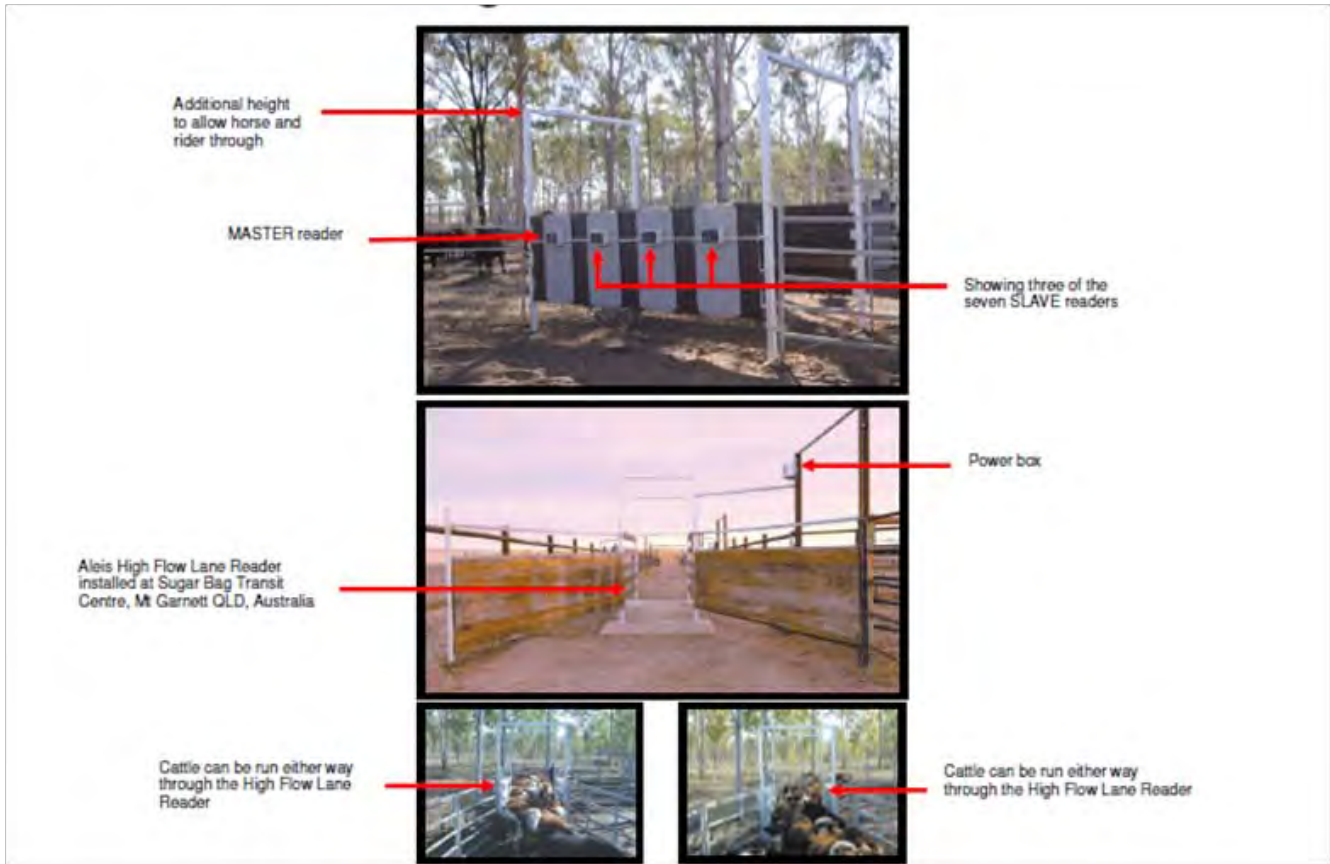
Diagram 2: The Multi Panel Scanning System used during the project to scan Regular Sales and Calf Sales.
