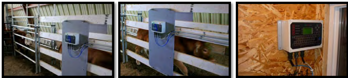
Picture 16, 17 and 18: Single alley scanning system (16) (17), Data box (18)
