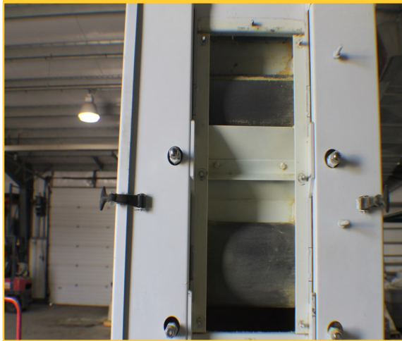
Figure 2. A roller mill can be used to reduce particle size of cereal grains intended for poultry
