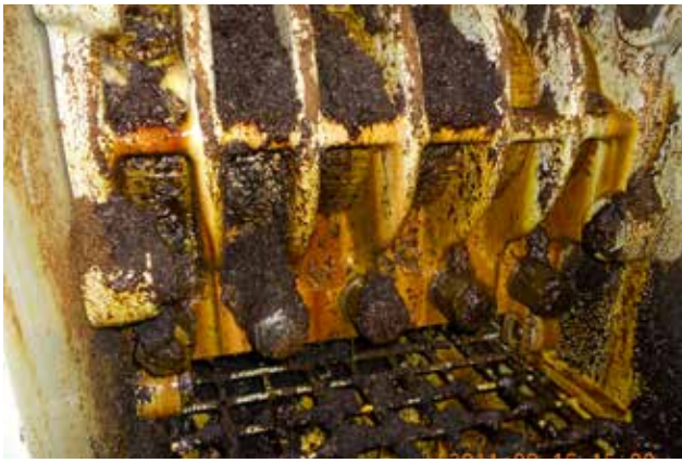
Figure 2. In an expeller press, greater pressure is exerted by a large screw expelling more oil out of the seed pressed against a barrel cage lined with bars.
