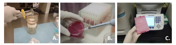
Water samples are filtered to trap bacteria on the surface of a membrane (A). The membrane is transferred to an agar medium that selects for *E. coli* growth (B). DNA is extracted from the isolated *E. coli* and supplies the material for DNA fingerprinting (C).
