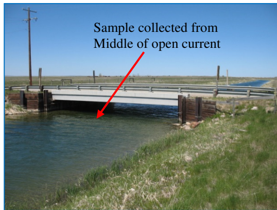
Figure 5. At each (a) canal outlet location, two samples should be taken, including (b) one from the middle of the open current and (c) and one near the shore. If an open current measurement is not possible, samples should be taken from both shores.
