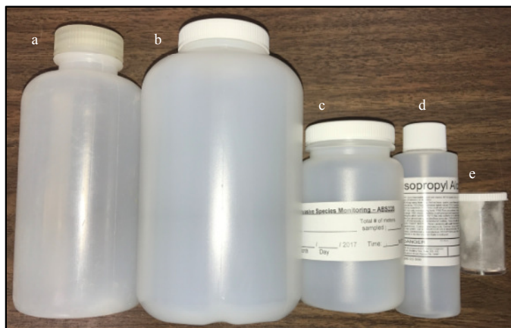
Figure 7. Veliger sampling equipment (a) Nalgene squirt bottle, (b) composite bottle, (c) sample bottle, (d) alcohol preservative, and (e) baking soda preservative.
