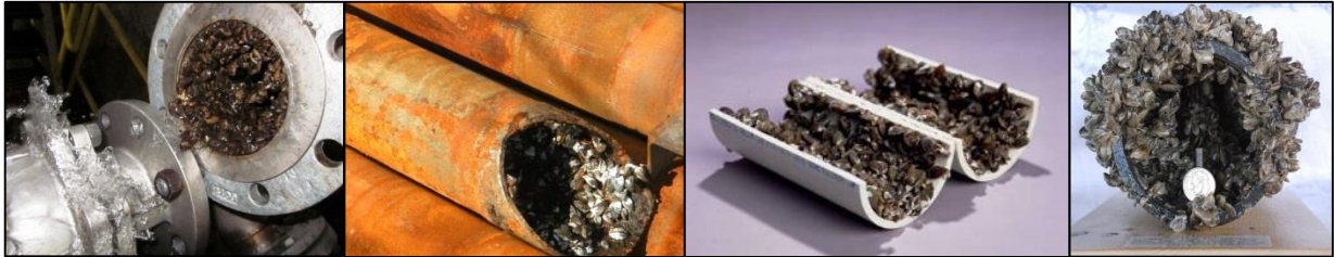
Figure 1. Examples of pipes fouled by invasive mussels.
