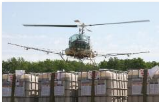
Helicopter used for aerial spraying (Note: mini-bulks with Btk)
