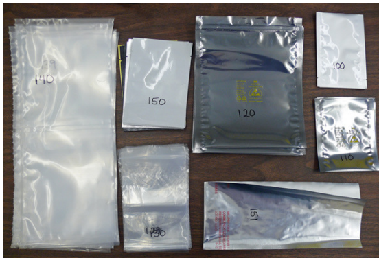
Bags to be tested for sealing. Zip-loc bags failed miserably!
