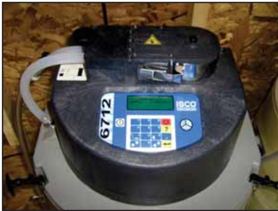
Figure 3.7. Model 6712 Isco automated water sampler.
