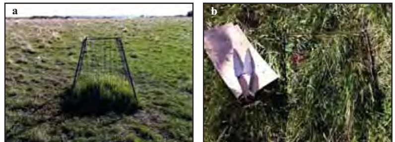
Figure 3.13. Views of a (a) production cage and (b) 0.25-m 2 frame used to delineate vegetation to be clipped.
