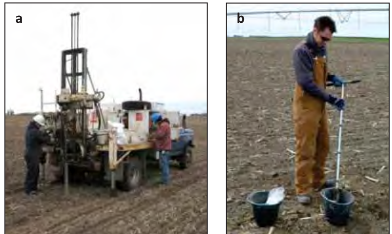
Figure 3.10. Soil sampling with (a) a truck-mounted coring unit, and (b) a Dutch auger.
