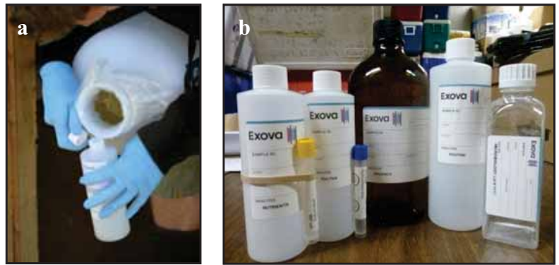
Figure 3.9. Water samples being (a) sub-sampled in the field and (b) bottles for specific lab analysis.
