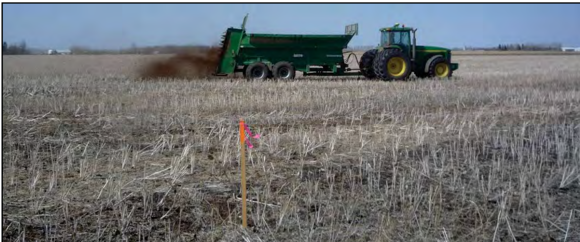
Figure 4.40. Manure application using a solid manure spreader with vertical beaters (Bunning Lowlander Widebody 230) at the West Field on April 15, 2010.
