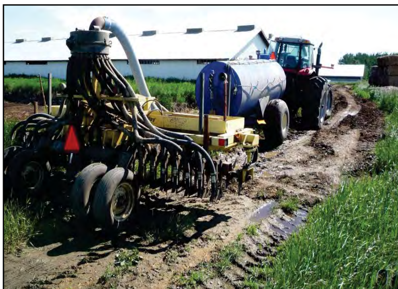
Figure 4.53. Manure applicator using drag tubes with AerWay® technology used for applying liquid dairy manure on alfalfa at the East Field site in July 2010 and 2011.
