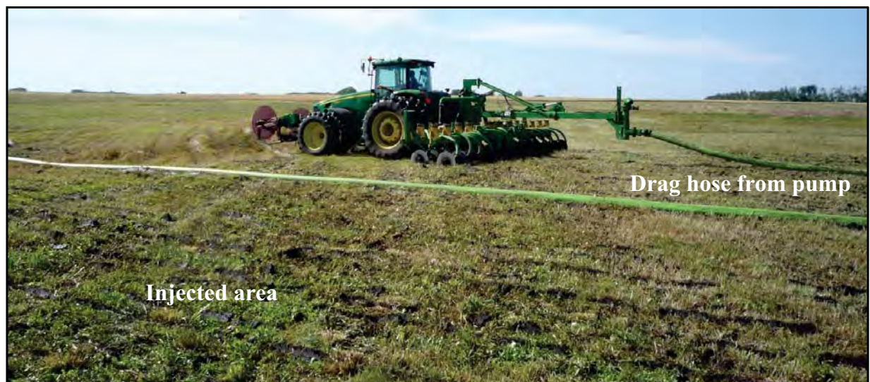
Figure 4.45. Tractor pulling a drag-hose system with disk openers used to inject manure in the southwest field at the North Field site on September 8, 2011.
