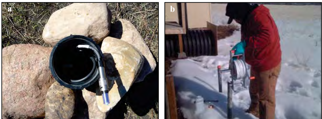
Figure 4.27. Measuring groundwater level using (a) a Level TROLL ® at Station 301 (outlet) and (b) a water level meter with depth sounder at Station 317 (Reference 1 site).
