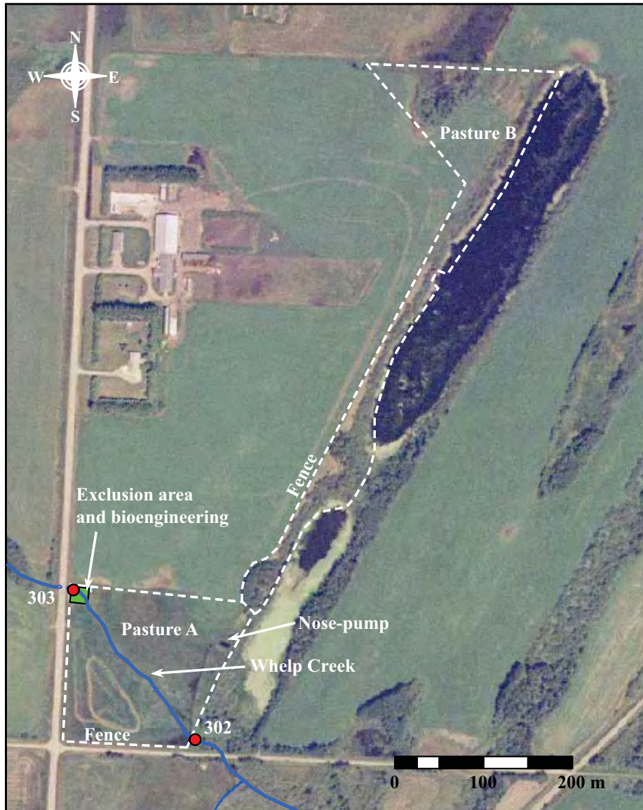
Figure 4.62. The North Pasture showing Whelp Creek, Pastures A and B, water monitoring stations (Station 302 and 303), the excluded and bioengineering area, and the nose-pump location.
