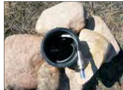
Levellogger in the groundwater well near the watershed outlet records water table height.
