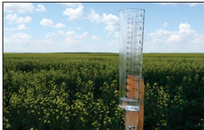
Figure 5.7. A rain gauge used to measure the volume of water applied by irrigation and precipitation at the Lower Little Bow River Field site.
