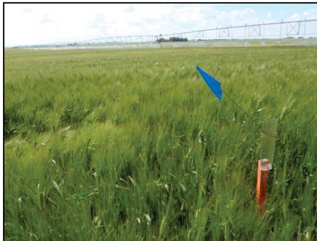
Figure 4.10. Manual rain gauge used to measure the amount of irrigation and rain received on the barley crop at the Battersea Drain Field site in 2010.
