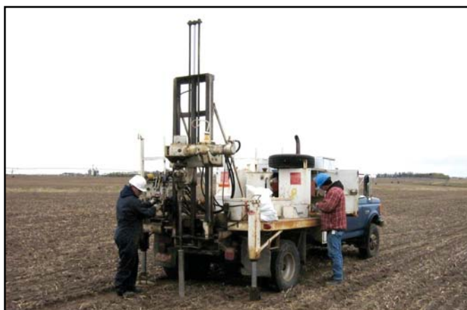
Figure 4.16. Moisture and texture soil sampling on April 27, 2010 at the Battersea Drain Field site.
