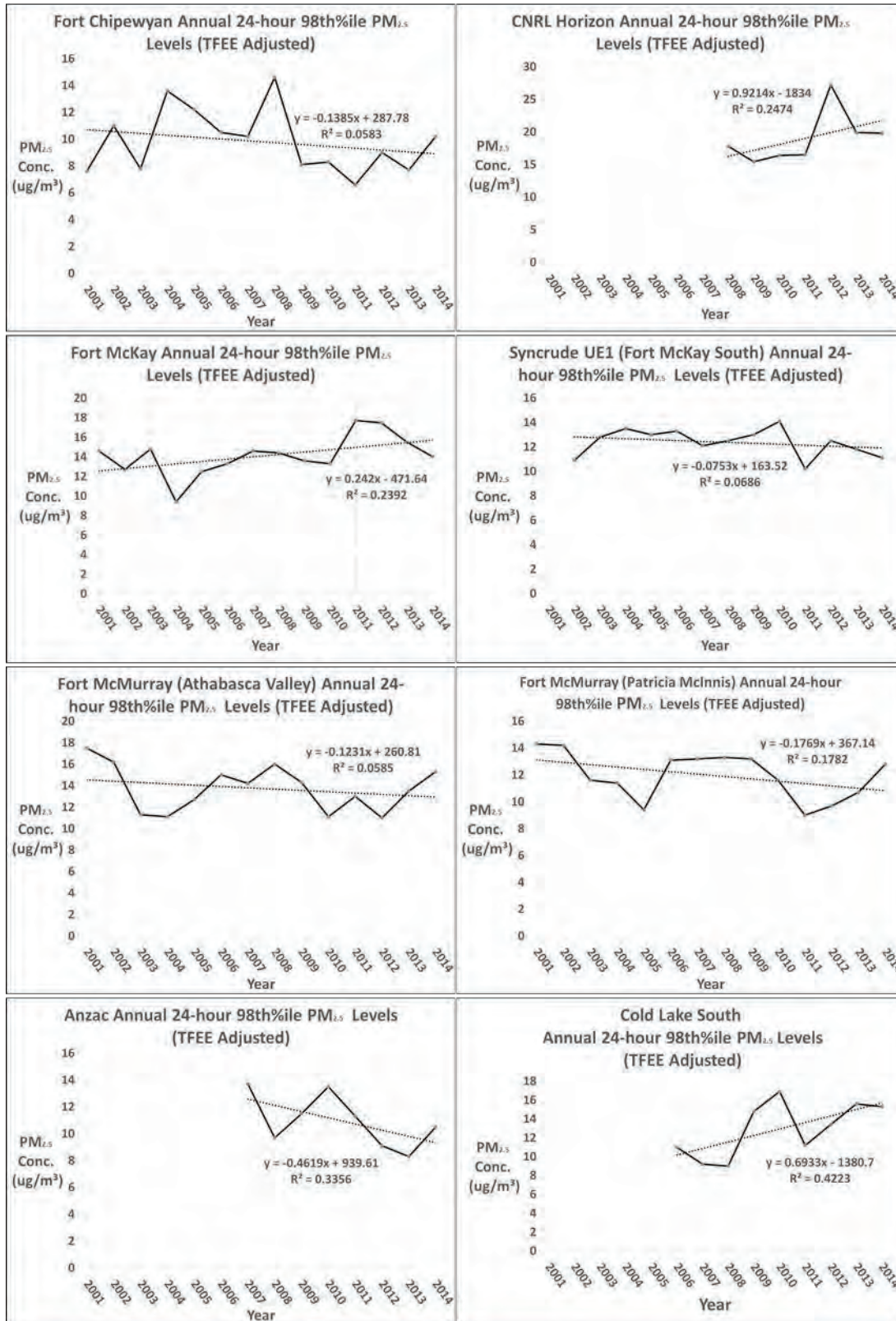
Figure 3: Plots and Linear Regression of the Annual 98 th Percentile PM 2.5 Concentration CWS/CAAQS Determination Values for the LAR Air Zone (note: vertical axis scale varies between plots)
