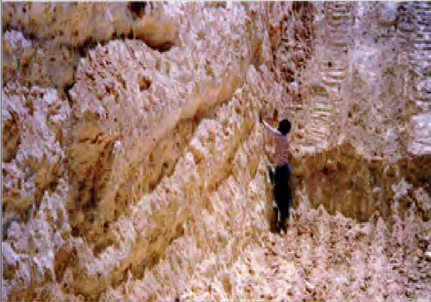
Figure 1. Excavated open trench in the Al Jalamid deposit showing 9.5m thick overburden of bioclastic dolomitic limestone and the top of the Thaniyat phosphorite member containing calcareous compact to semi-friable phosphorite with 25% P_2O_5 (level with figures waist).
