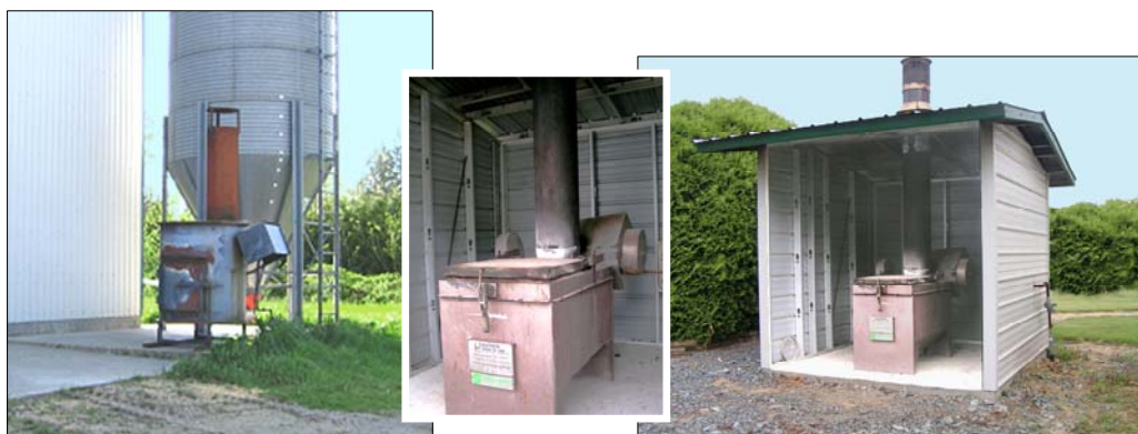
Figure 26 Examples of a Stationary On-farm Incinerator
