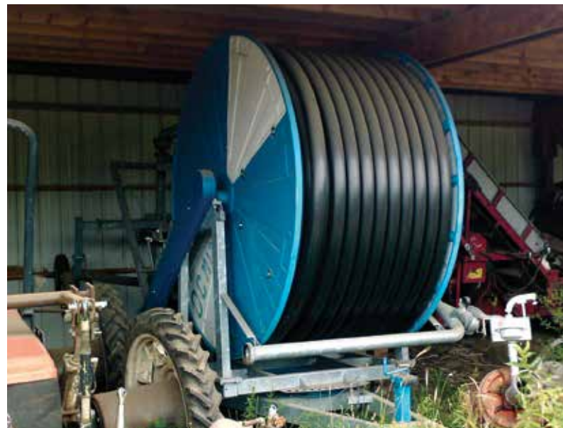
Travelling volume gun and reel system Photo: Robert Spencer
