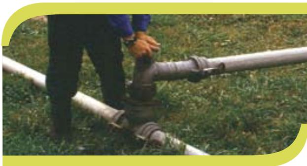
To stop a manure pipeline spill, shut down pumps and valves.
